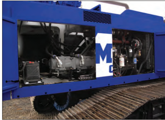
Large access doors, spacious machinery compartments simplify preventative maintenance and service of the crane.
